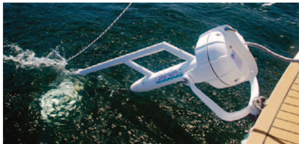
The Sail Gen from Eclectic Energy has an adjustable trim tab that keeps the unit at the right depth and makes recovery easier
