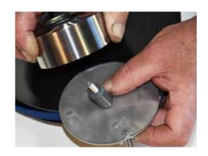
9: At this point you no longer need to secure the coil spring with the palm of your hand. Do not move the assembly until the next step is completed to prevent the spring coil from becoming dislodged.
