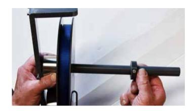
13: Push the axle through hub and guide arm until the retaining collar is seated against the end plate of the belt reel.
