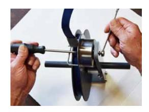
15: Use a feeler gauge to set the retaining collar to provide a clearance of 1mm (3/64 in).
