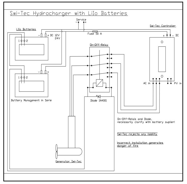
The charge controller will placed and fixed with four screws in a dry compartment in the vicinity of the batteries in a matter that you can see good the digital display. The battery cables should be as short as possible. Plus on the connector **"Batt** +" and with a red cable on the plus of the battery and the black cable from the "Batt –". A 40 Amp fuse in the red wire protects the Hydro Charger Deluxe in case of a short circuit of the batteries.
